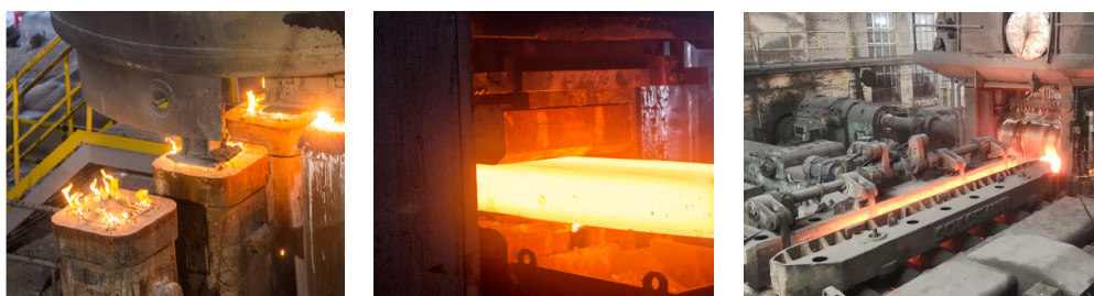
Casting, forging and blooming operations carried out at Tubacex facilities
